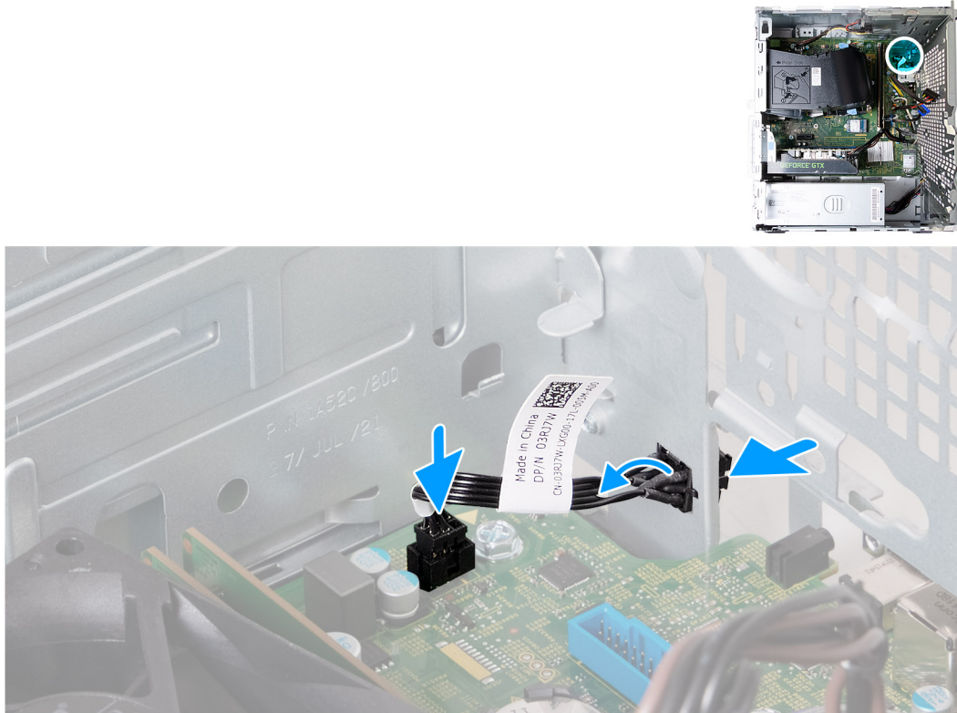
Figure 27. Installing the power button
