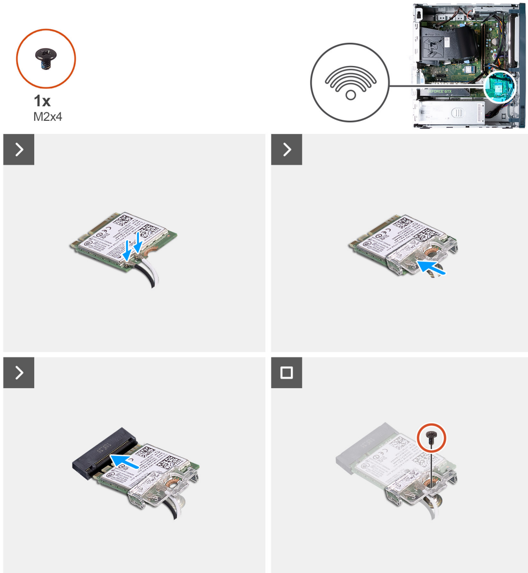
Figure 21. Installing the wireless card
