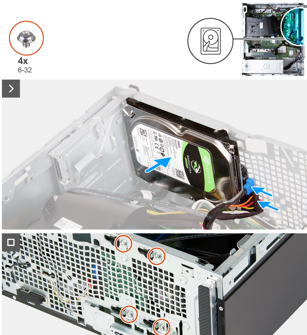
Figure 25. Installing the hard drive
