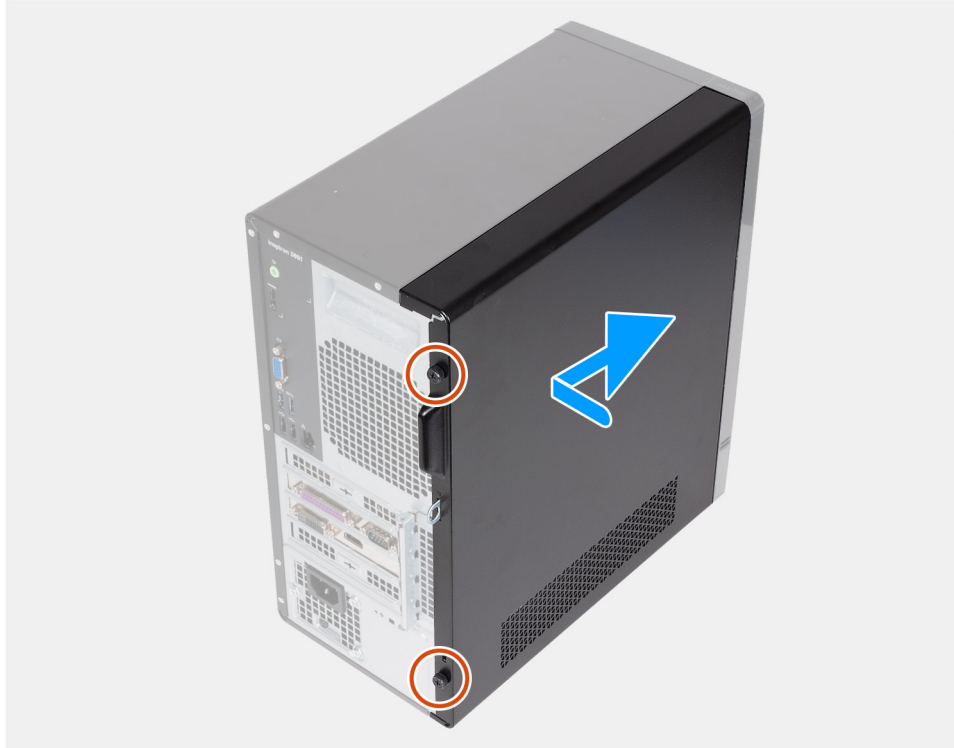
Figure 13. Installing the left-side cover
