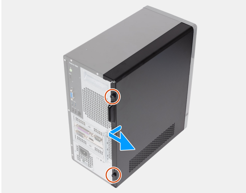
Figure 12. Removing the left-side cover
