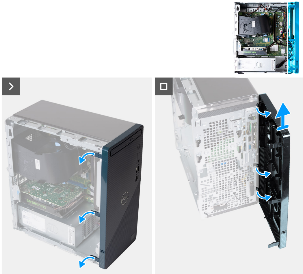
Figure 14. Removing the front cover
