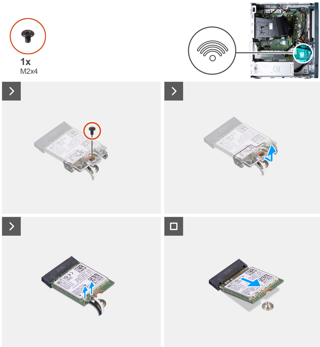
Figure 20. Removing the wireless card
